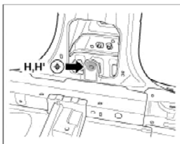
Front seatbelt retractor mounting hole (ø12)
