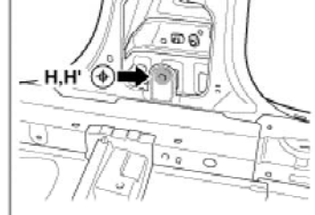
Front seat belt retractor mounting Hole (ø13)
