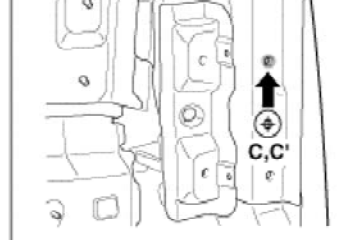
Cowl crossbar mounting hole (ø9)
