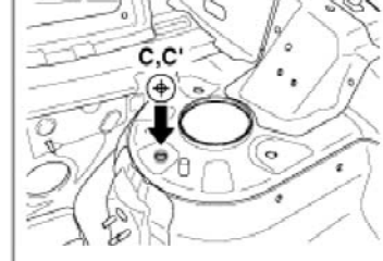
Front suspension mounting hole (ø11)
