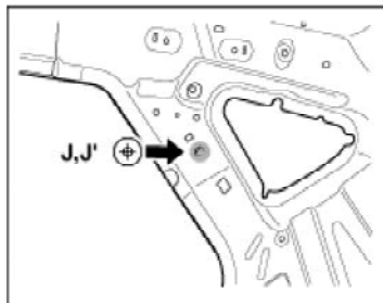
Rear seatbelt anchor mounting hole (ø14.5)
